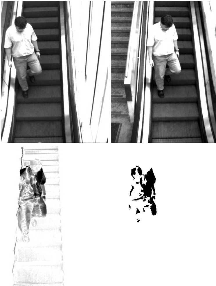
Fig. 3. Images and results for a person on a staircase: left and right images, absolute differences of left image warped to right image, and pyramid-based segmentation result
