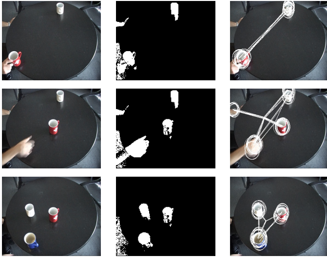
Fig. 4. Three frames from the dining table sequence. Column one shows the input frame, column two the foreground/background segmentation, and column three the top 2% of the 1000 configuration hypotheses.
