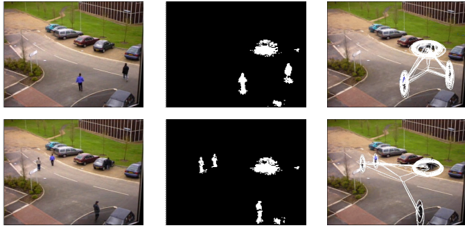
Fig. 2. Two frames from the PETS2000 dataset. Column one shows the input frame, column two the foreground/background segmentation, and column three the top 1% of the 5000 configuration hypotheses.
