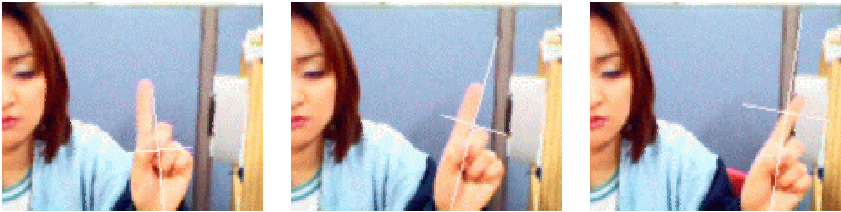
Fig. 4. Growing the search window in the CAMSHIFT algorithm
