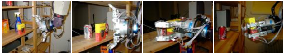
Fig. 5. A few example images during servoing onto and grasping a package of raisins.
