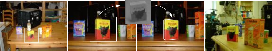
Fig. 6. The basic idea of our approach: after the object is recognized, 2D tracking is used to approach the object. After that, the appearance based approach followed by a local fitting stage is used to estimate the current pose of the object. After that, simple grasping can be performed.
