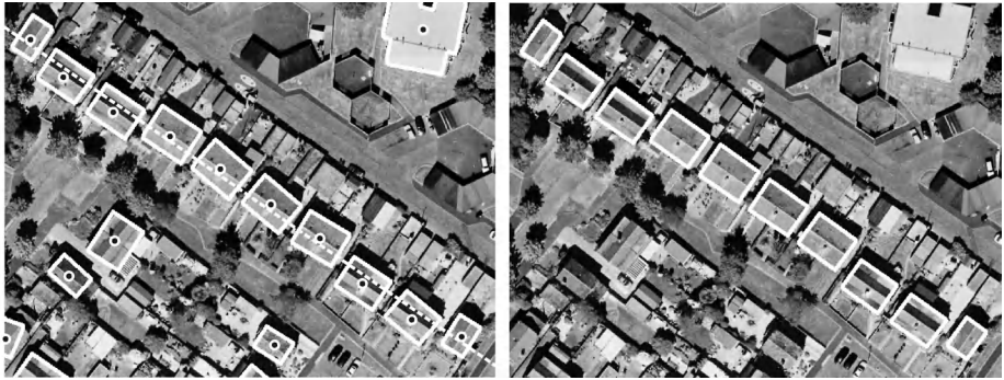
Fig. 5. Reconstructed buildings with marked centers of gravity and row of buildings (left), buildings after orientation enhancement (right)
