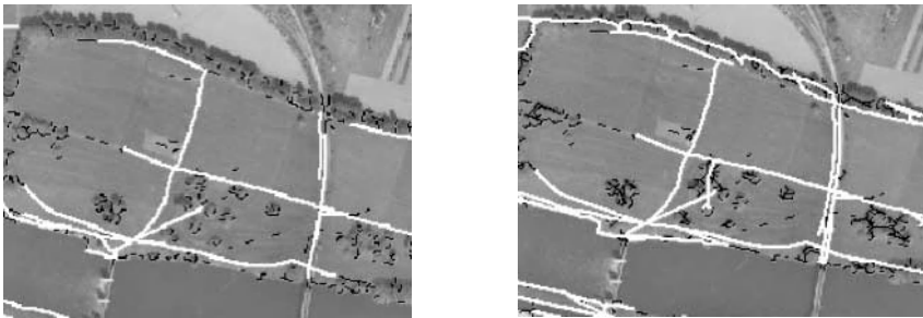
Fig. 6. Results of the road extraction without the support of trees depicted in the left image, the image on the right side shows the results of the road extraction algorithm together with rows of trees.
